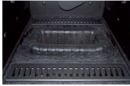
Burner and ashes extractor
