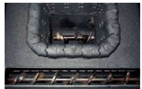
Ash extractor: combustion chamber
