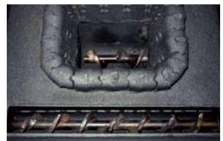
Ash extraction: combustion chamber
